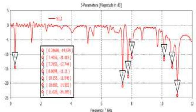
**Figure 7:** ON state S<sub>11</sub> scattering parameter
