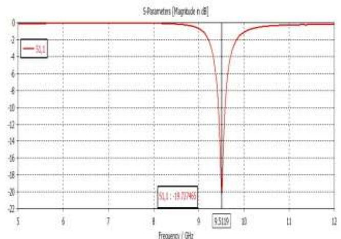
**Figure 3:**  $S_{11}$  Vs Frequency graph for OFF state
