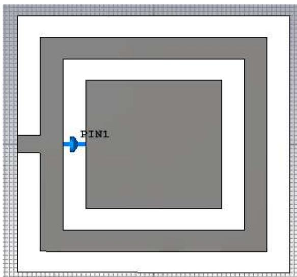
**Figure 5:** Design 2 with PIN Diode
