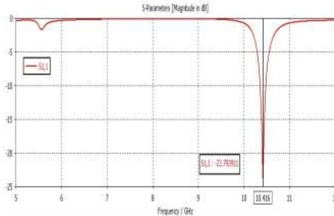
**Figure 4:** S<sub>11</sub> Vs Frequency graph for ON state
