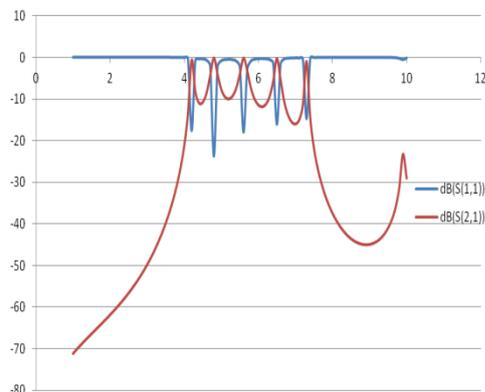
**Fig.3:** S<sub>11</sub> and S<sub>21</sub> plot with U-Shaped DGS
