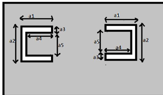
Fig 2: Bottom view of Hairpin bandpass filter
