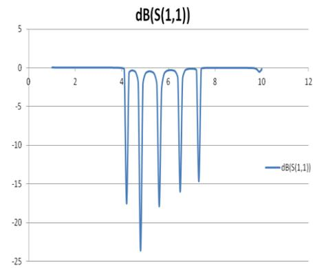
**Fig.4:** S<sub>11</sub> plot with U-Shaped DGS
