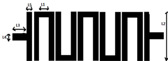
Fig. 1: Top view of Hairpin bandpass filter.
