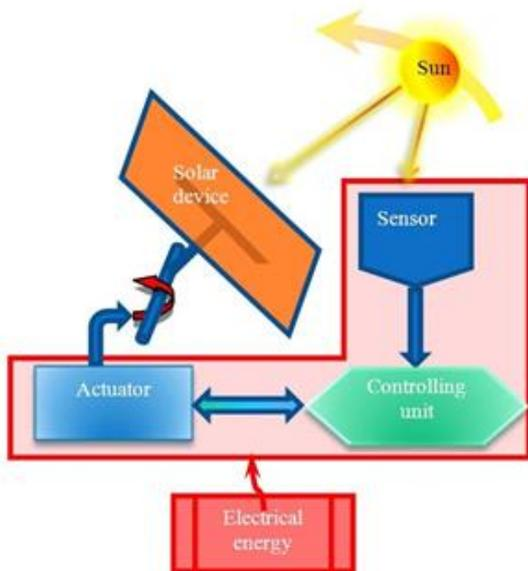
**Figure 1.** Working elements of a typical currently existing sun tracking mechanism
