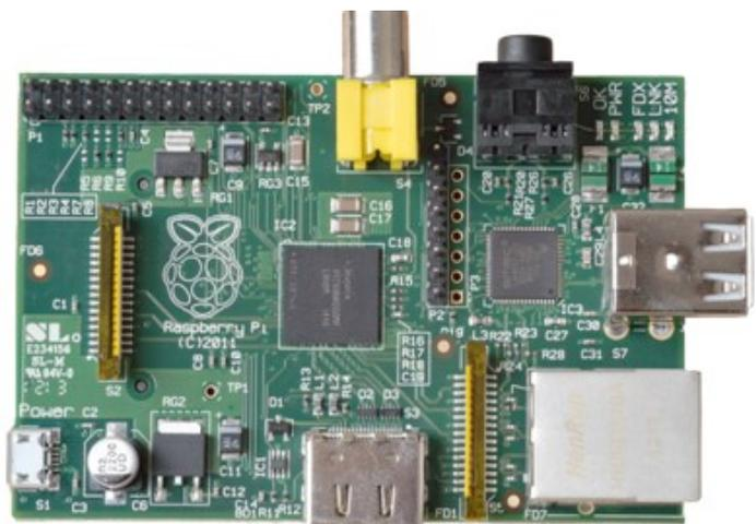
Fig.3 Raspberry pi board
