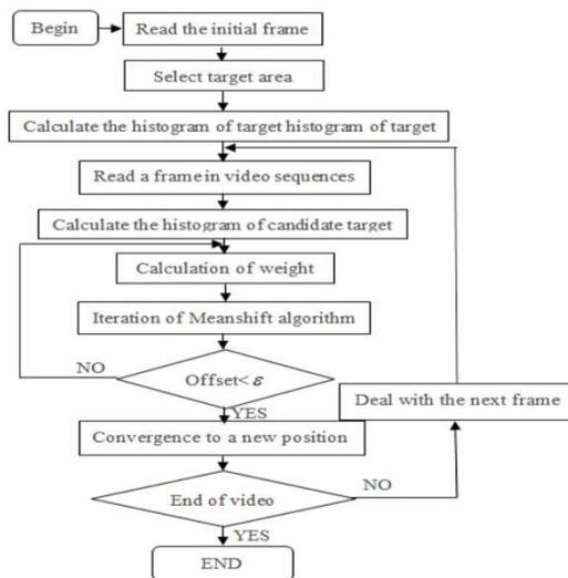
Figure 2. Detailed Flow Diagram
