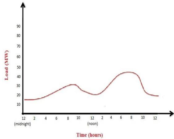
Figure: A typical daily load curve
