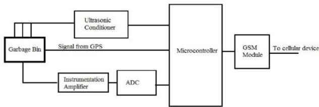
**Figure 1.** Block diagram for Smart Garbage Bin
