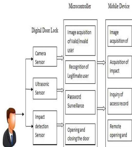
Figure 1. Structure of system
