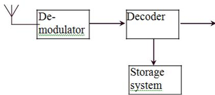
Fig.6 Receiver Process
