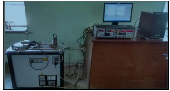
Figure 6: Setup of Pin on Disc Machine
