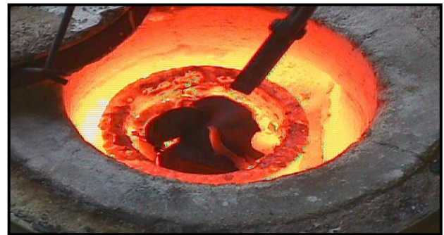
Figure 1. Set-up of Stir Casting
