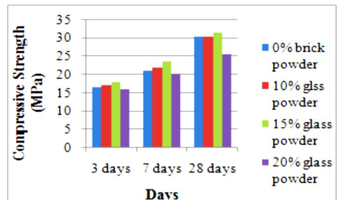
**COMPARISON OF COMPRESSIVE STRENGTH OF M-20 MIX FOR DIFFERENT PERCENTAGE OF GLASS POWDER**
