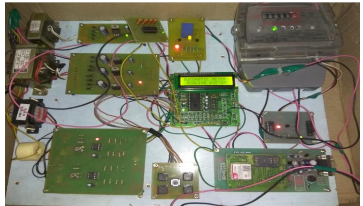
Figure 4: Hardware Implementation of Proposed System
