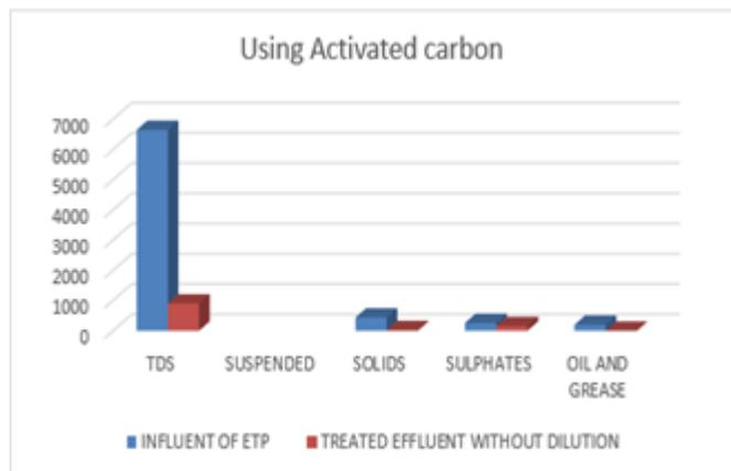
Graph. 4 graph of parameters using activated carbon
