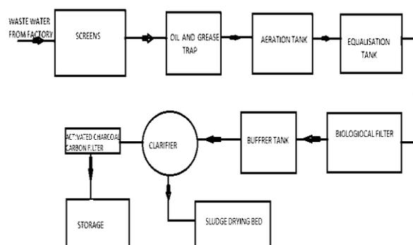
Figure 2. Flow Chart of Effluent Treatment Plant
