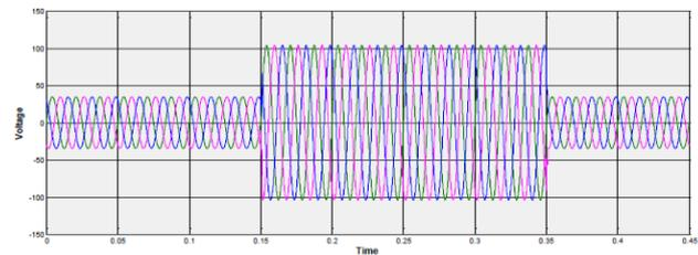
Figure 5(c) Load voltages during sag
