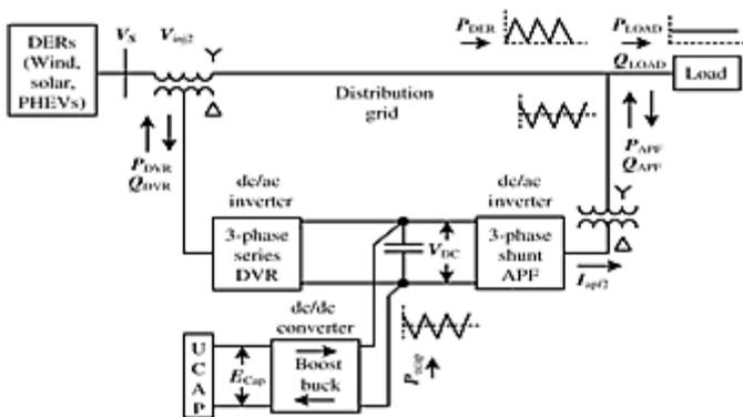
Figure 2 : One-line diagram of power conditioner with UCAP energy storage
