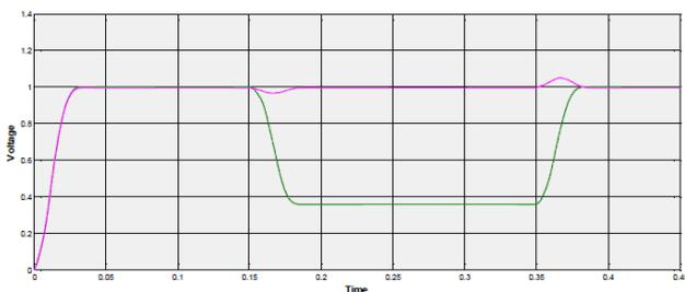
Figure 5(a). Source and load rms voltages during sag
