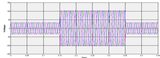
Figure 5(c) Load voltages during sag
