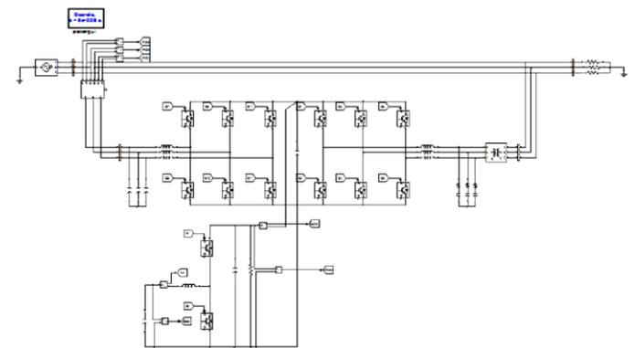
Figure 4. Simulink Model of power conditioner with UCAP energy storage
