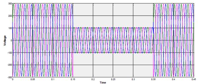
Figure 5(b). Source voltages during sag
