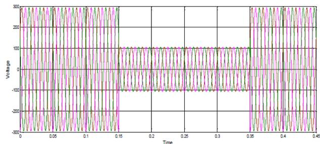
Figure 5(d) Source voltages of simple capacitor during sag
