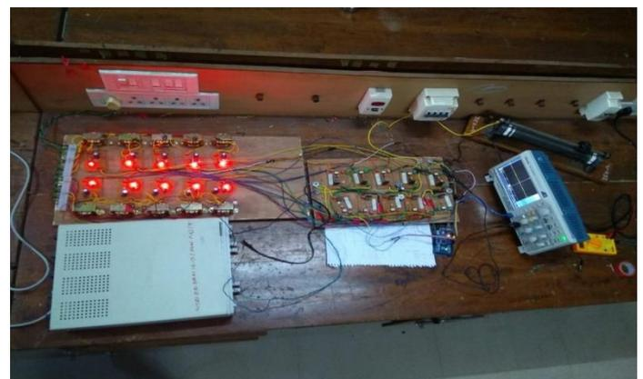
Fig. 5 Hardware setup of multilevel inverter
