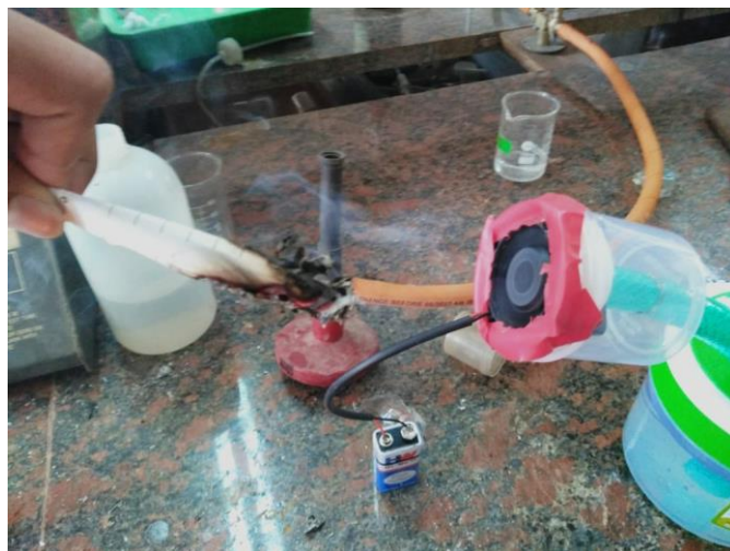
Figure 1. The air is sucked through intake fan.
