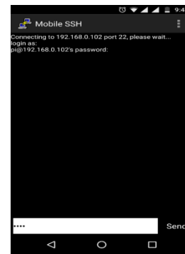
Figure 11. Mobile SSH connecting to Raspberry PI using PI id and password
