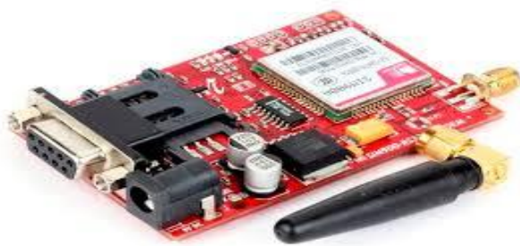
Figure 5. SIM800L GSM/GPRS/GPS module
