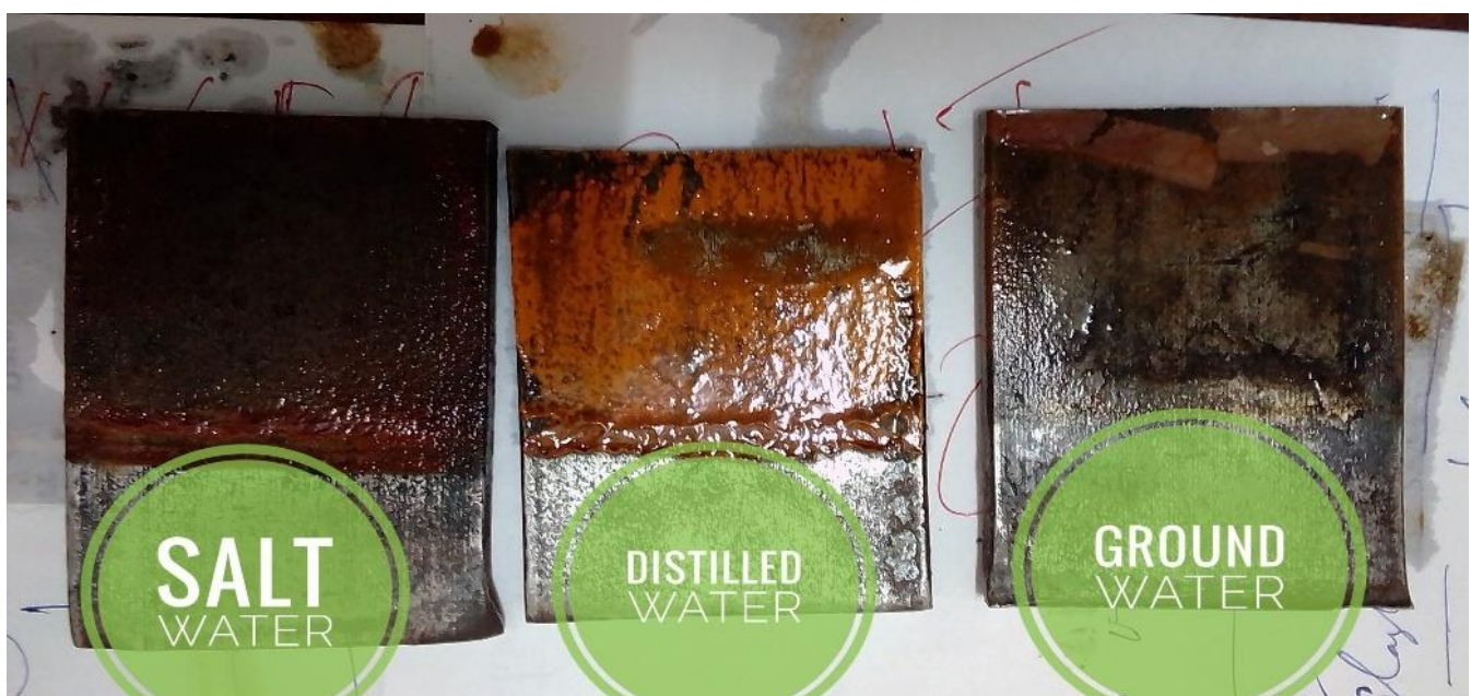
Figure 1. picture of water samples after 24 hrs.
