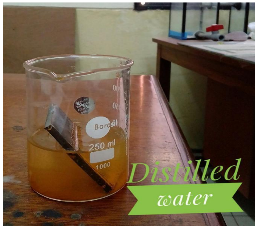
Figure 3. Metal in distilled water after 48 hrs
