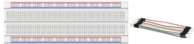
Figure 7. Breadboard and Jump wires
