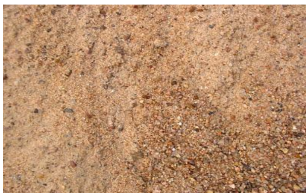
Figure 1. Fine aggregate – Sand
