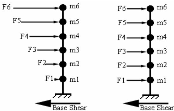
Figure 1. Conventional lateral load distribution
