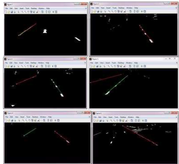
Figure 8. Lane detection results by Hough transform
