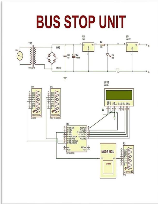
**Figure 3 :** Circuit Schematic of Bus Stop Unit.
