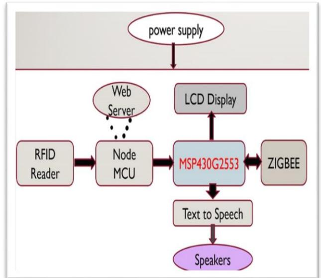
**Figure 1 :** Block diagram of bus stop unit.
