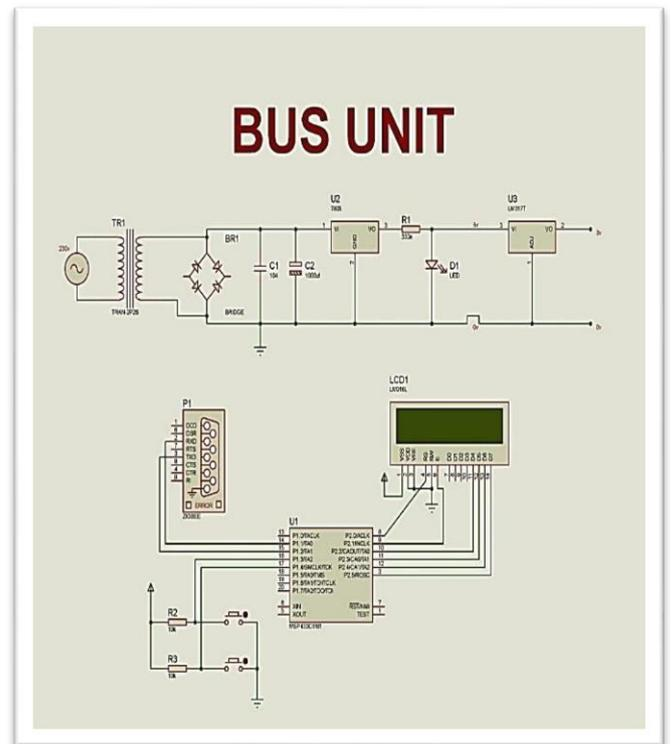
**Figure 4 :** Circuit schematic of bus unit.
