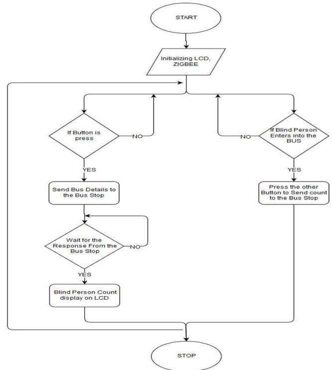
Figure 11b. flow chart of bus unit.
