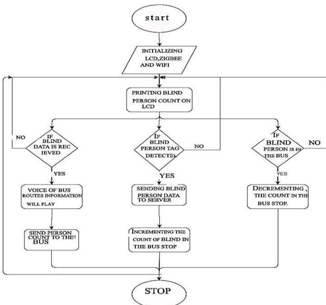
Figure 11a : flow chart for bus stop unit.
