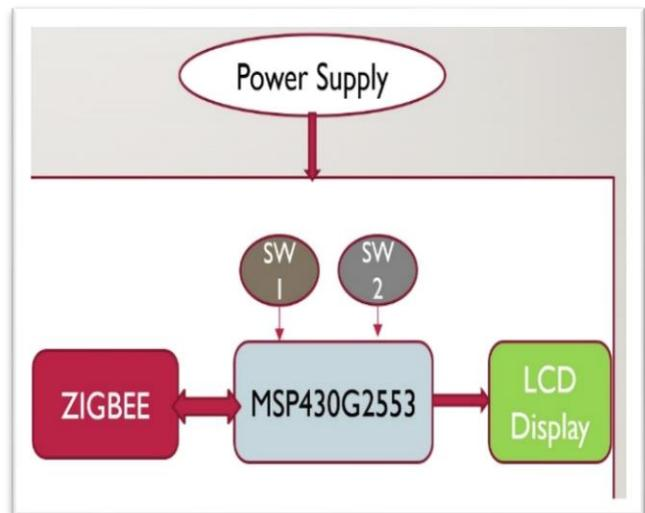
**Figure 2 :** Block diagram of bus unit.
