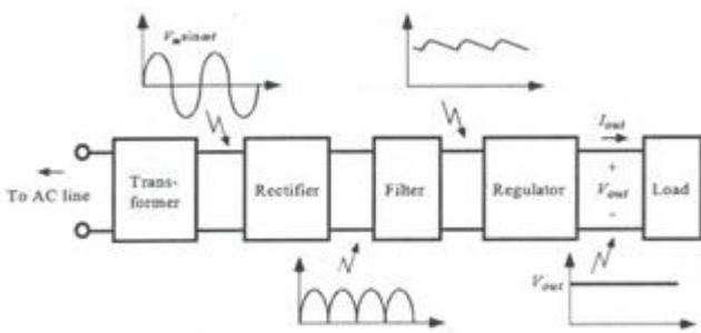
Components of a regulated power supply
