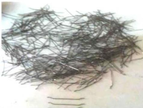
Fig 1: Steel fibre
