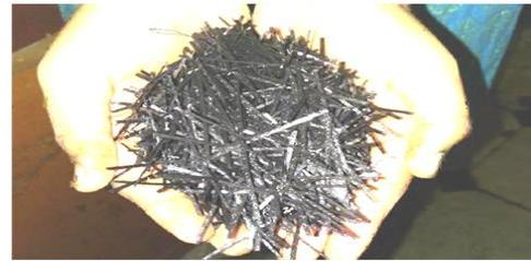
Fig 2: Polyolefin fibre
