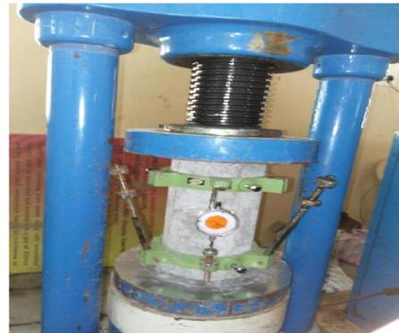
Fig 2: Testing of Cylindrical mould
