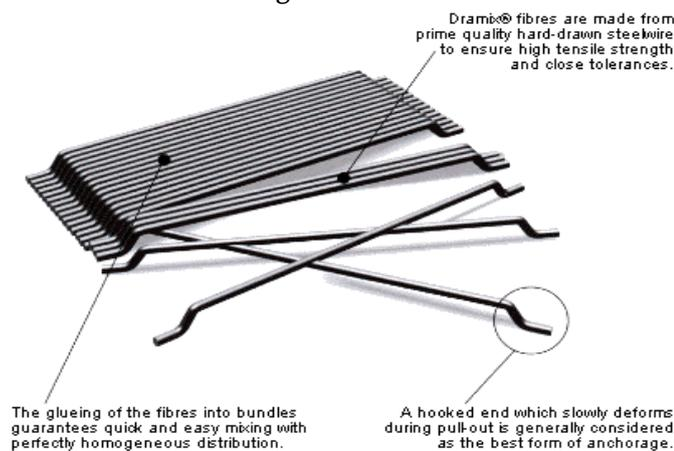
**Figure 2.1 :** The figure shows the general view of steel fiber
