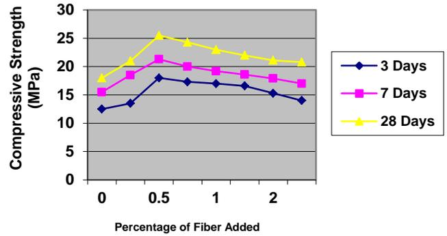
**Figure 4.2:** Graph shows the compressive strength of M<sub>20</sub> grade concrete with and without polypropylene fibre
