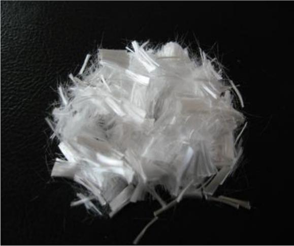
**Figure 2.2 :** The figure shows the general view of polypropylene fiber
