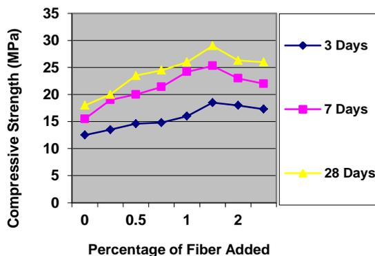
**Figure 4.1 :** Graph showing the compressive strength of M<sub>20</sub> grade concrete with and without steel fibre
