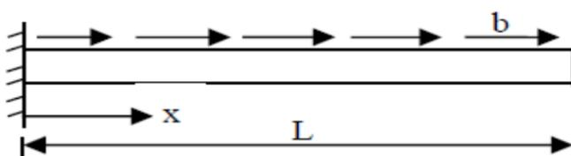
Figure 1: Axially loaded bar
