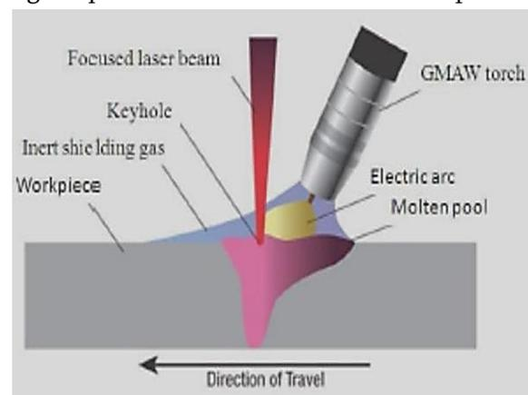
Figure 1. Gas Metal Arc Welding
