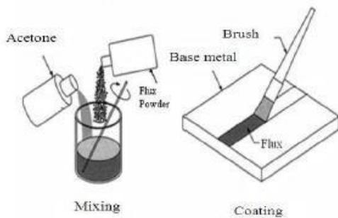
Method of applying flux
