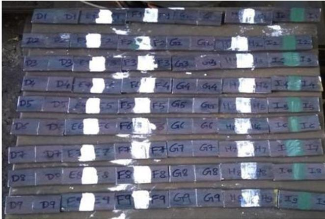
Step 3-To ensure highly smooth contact surface the surfaces are then buffed through buffing wheel.
