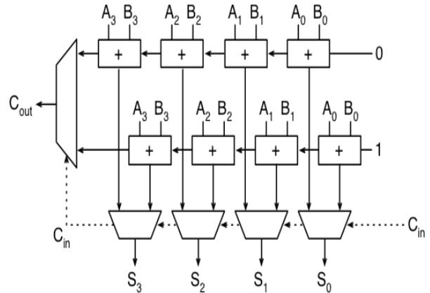
**Figure 2.** 4-bit Carry Select Adder
