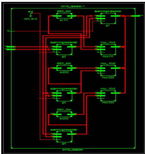
Figure 4. Block Diagram and RTL Schematic of CSA With STA
