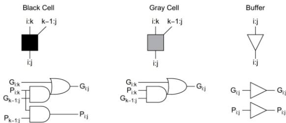
**Figure 1.** Various cells used within carry generation stage
