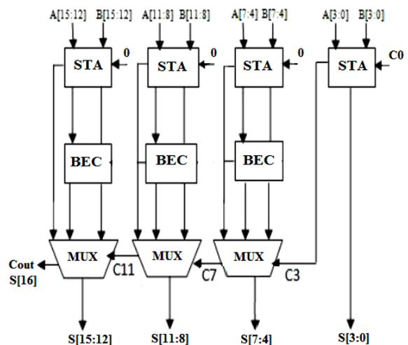
Fig. 3 Proposed 16-bit CSLA with STA
