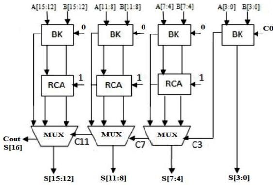
Figure 4. Carry Select adder Using Brent Kung Adder
