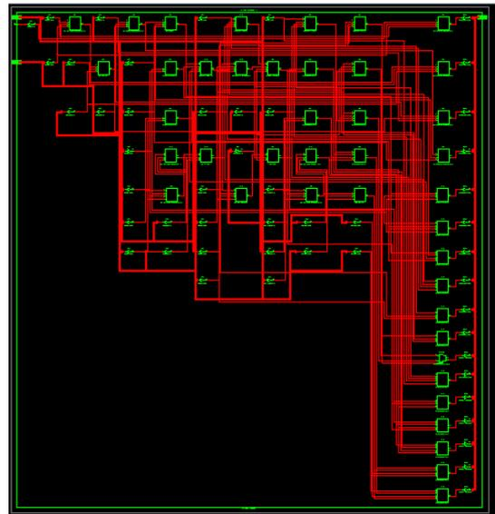
Figure 8. Technology schematic Of Proposed CSA with STA
