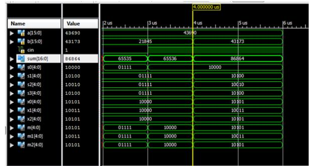
Figure 9. Simulation output of proposed CSA with STA
