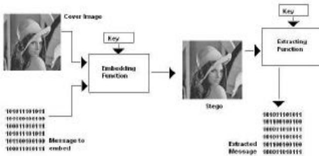
Figure 2. Steganography procedure
