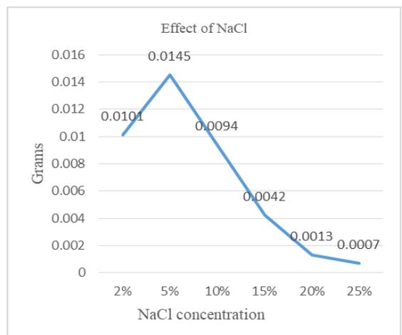
**Fig. 7 :** Effect of NaCl on production of PHB
