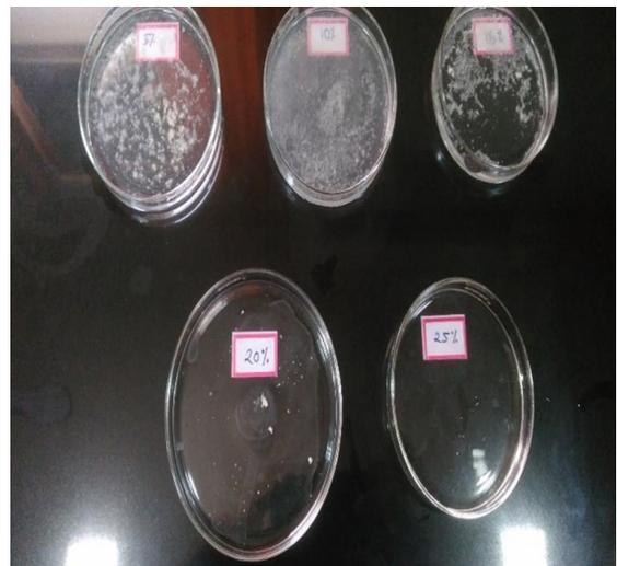
**Fig. 6 :** Extracted PHB at different NaCl concentration
