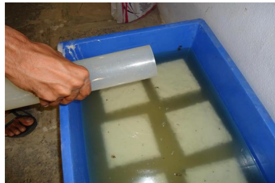
Pouring of acid to maintain constant acidity at regular interval of 5 days
