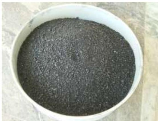
**Fig 1.** Appearance of copper slag sample
