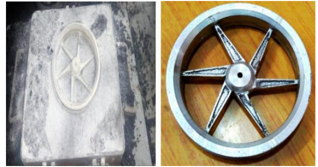
Fig 11 Proto type of Al6061 Alloy Wheel
