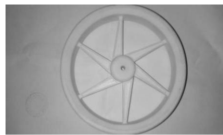
Fig 2. Pattern made from FDM with ABS material
