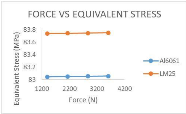
Fig. 9 Force vs Equivalent stress.
