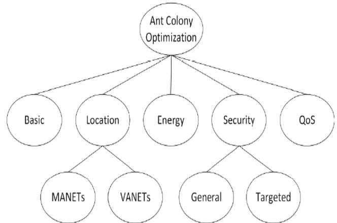
**Figure 1.** Types of ACO based routing protocols in MANET
