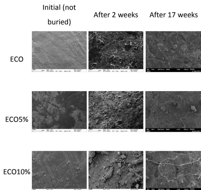
Figure 2: SEM photomicrographs of the Ecobras™/coconut fiber composite samples in the degradation test by burial in simulated soil, according to number of weeks. ECO: Ecobras™ free green coconut rush fiber samples; ECO5%: Ecobras™ composite samples with 5% coconut fiber; ECO10%: Ecobras™ composite samples with 10% coconut fiber
