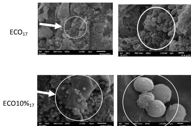
Figure 3: SEM micrographs of the Ecobras™ and ECO10% composites samples after 17 weeks of biodegradation burial test
