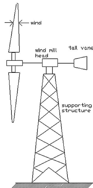
Figure 4 : Horizontal – Axial Machines
