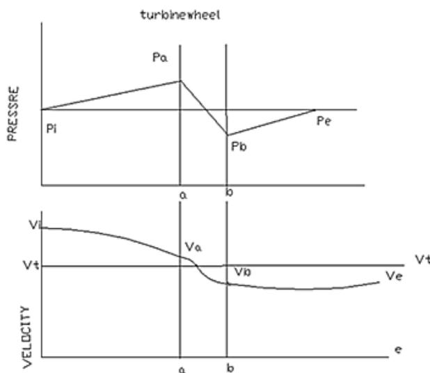
**Figure 1:** Line diagram of Turbine wheel
