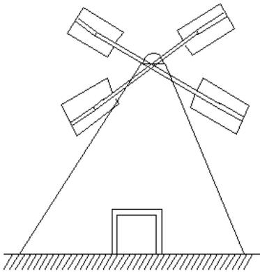
**Figure 6 :** Horizontal axis wind mill-Dutch type
