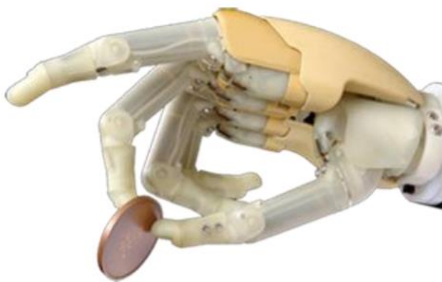
Figure 4. iLimb Hand (Arthur Finnieston Prosthetics + Orthotics, 2012)
