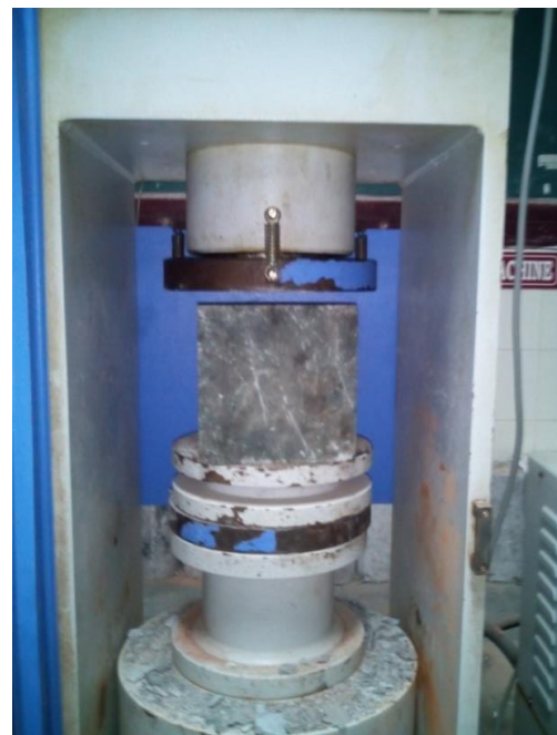
Fig 4.9.1 Testing of Compressive Strength of Cube
