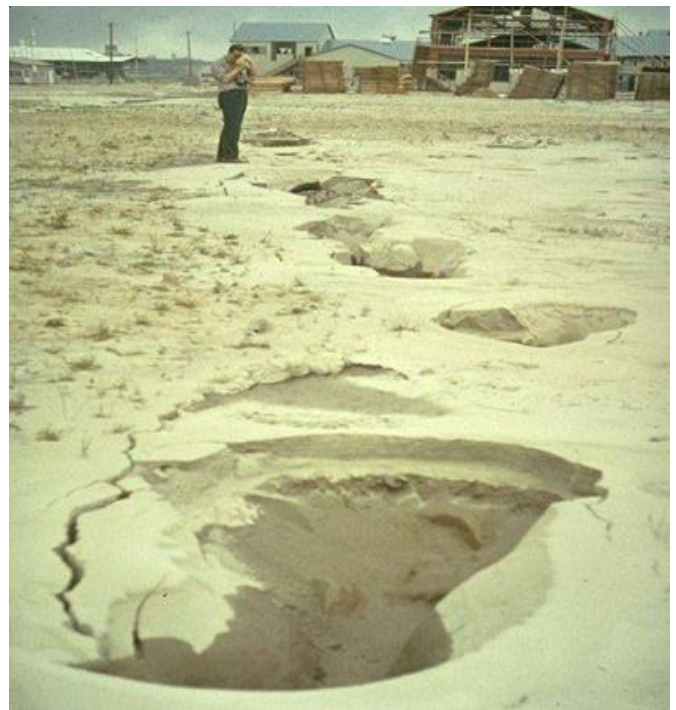
Fig.1.2 A remarkable ground failure occurred near the Shinano river bank in Niigata earthquake
