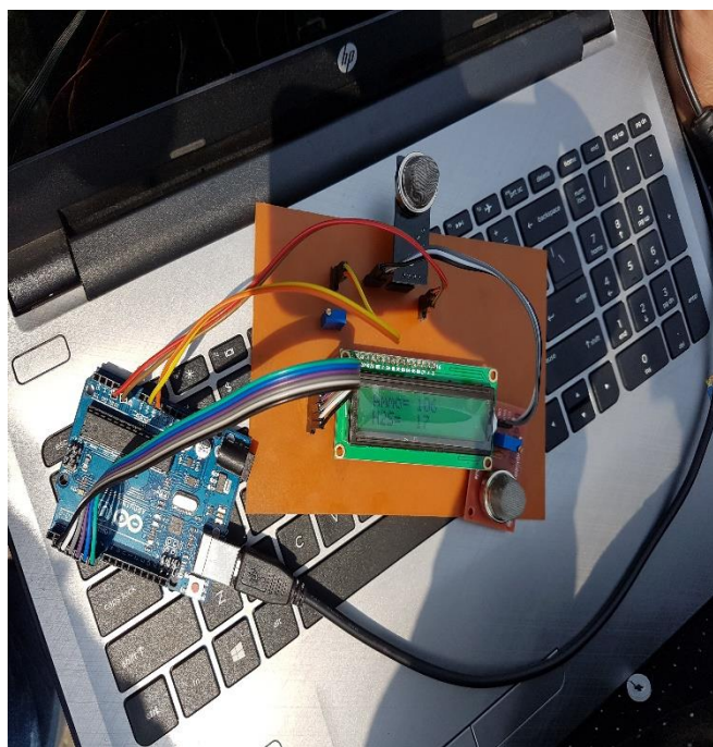
Fig.1 Arduino Uno based odor sensory measurement system
