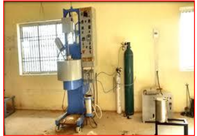
Fig. 4: A stir casting setup, consist of a Coke fired Furnace and a stirrer assembly, which was used to synthesize the composite.
