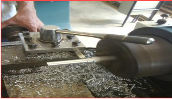
Fig 5 Turning operation carrying on lathe
