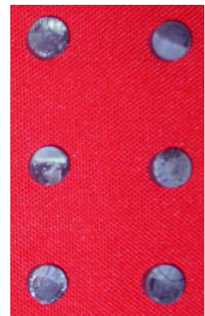
Figure 3: EDMed wear specimen
