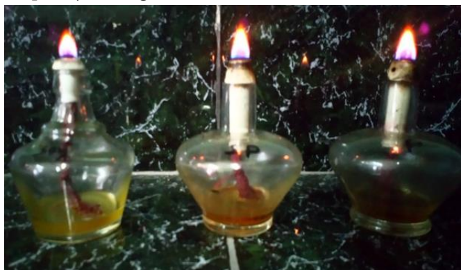
Figure-3: Flame height and color of biodiesel derived from soybean, super and palm oil (from left to right)
