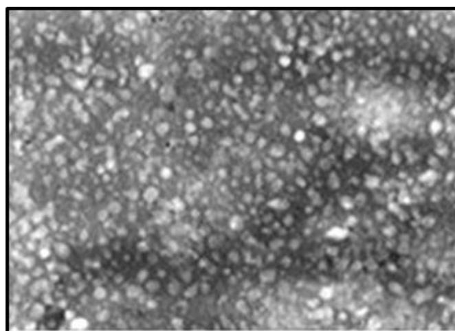
**Figure 7.** TEM analysis of copper nanoparticles
