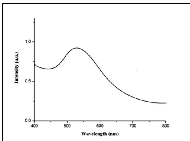
**Figure 3.** UV-visible spectra of gold nanoparticles
