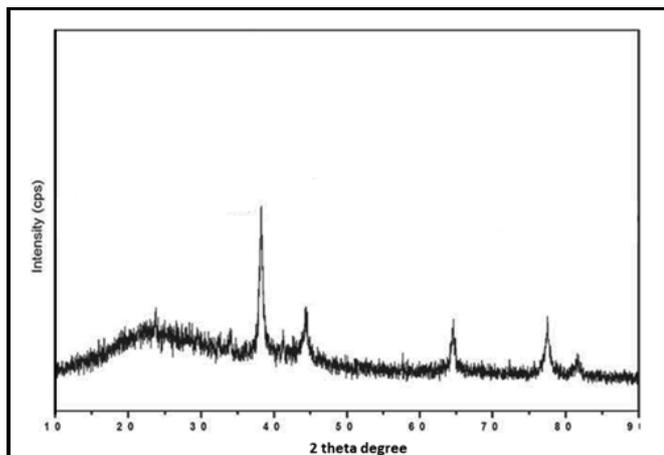
**Figure 5.** XRD pattern of gold nanoparticles synthesized from an extract
