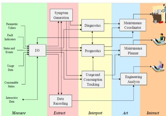
**Figure 1.** Basic Structure of IVHM
