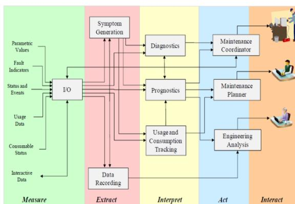
**Figure 1.** Basic Structure of IVHM
