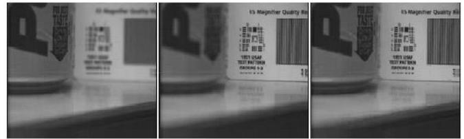
(a). Image 1 (focus on left) (b). Image 2 (focus on right) (c). Fused image (all focus) \*
