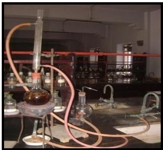
Figure 2: Photograph of experimental set up for obtaining plant extract using reflux condenser
