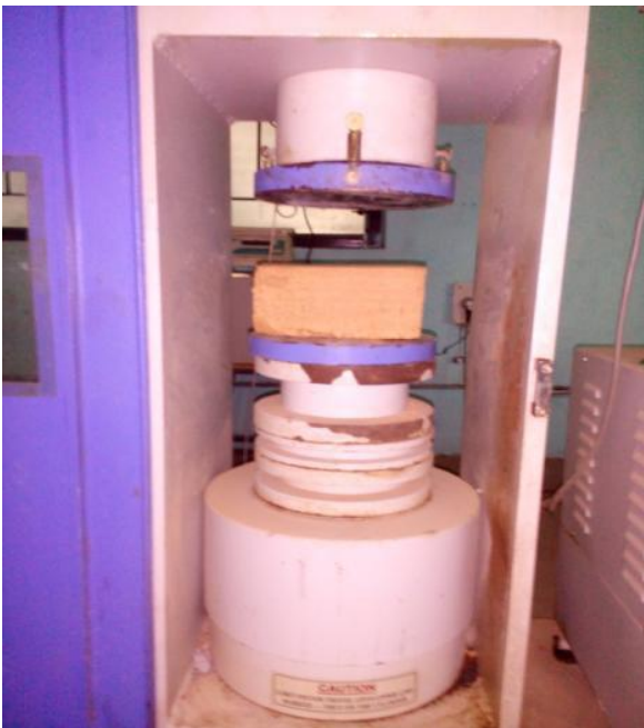
Figure 4: Compression test on Stabilized Brick
