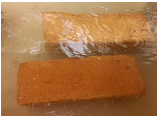
Figure 5: Immersion Test on Stabilized Bricks
