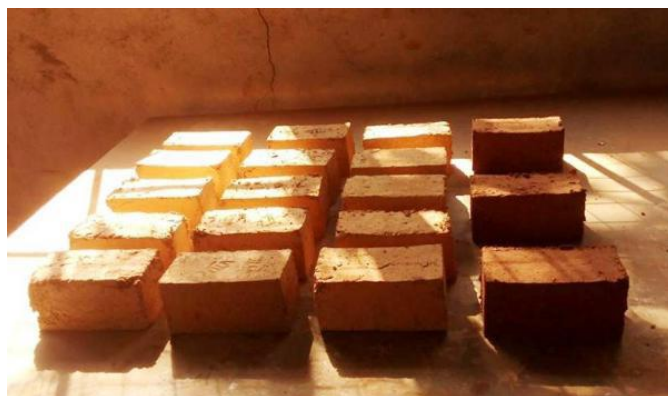
Figure 3: Stabilized earth blocks kept for drying
