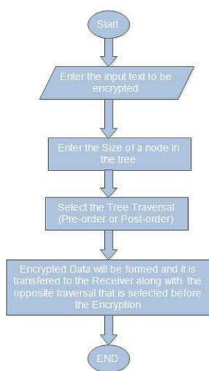
**Figure 5 : Steps @ sender for Encryption**
