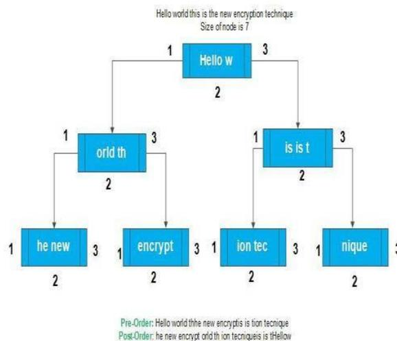
**Figure 6 : Steps @ sender for Encryption**
